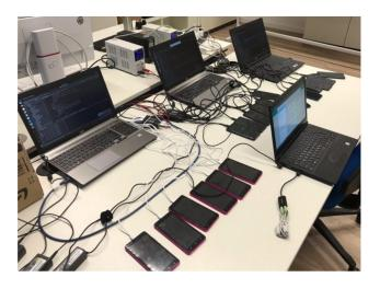
**Figure 2.** Case scenario hardware setup in the first experiment. Each device set (A, B, and C) consists of six devices (1–6) and each device set is controlled by a dedicated laptop (from left to right: Person C, XGody S20 Lite; Person A, Alcatel 1SE; and Person B, Samsung Galaxy A40). One additional laptop (in front) controls the FSM and generates voice messages. The dedicated power supply (in the back) powers the USB hubs and thus charges the devices.
