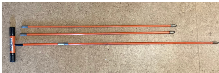
Figure 4. Van Walt peat probes (75 cm lengths) with steel tips—ideal for boat deployment in the search protocol suggested.
