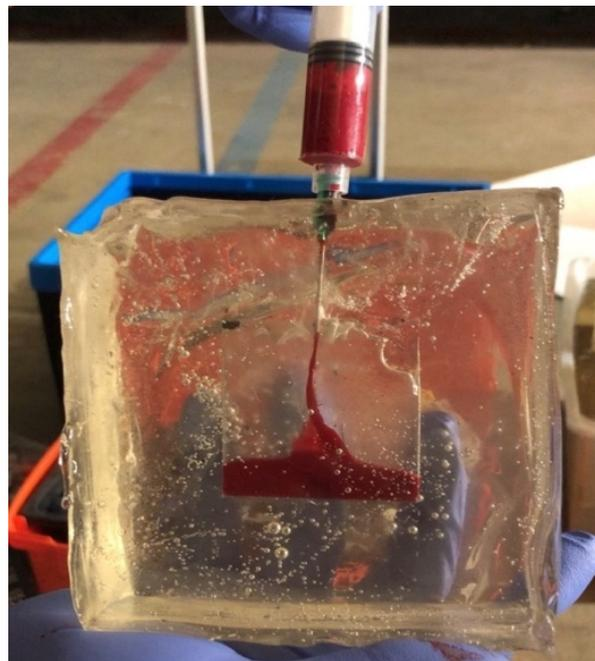
**Figure 7.** Syringe injecting the 6 mL of blood into the enclosed chamber of the ballistic gel.
