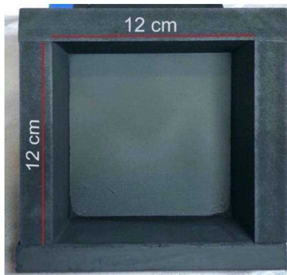
**Figure 1.** A  $12 \times 12$  cm wooden frame sprayed with heat enamel spray paint to make ballistic gel mould.
