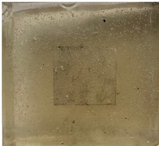
**Figure 3.** An enclosed ballistic gel mould with the closed chamber pocket (centre darker square).
