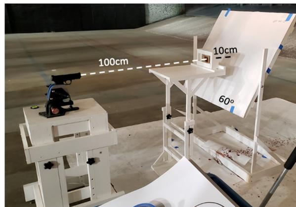
**Figure 5.** Overall methodology in situ from trial 10 cm at 60°, paper target rig (**far right**), gel block stand (**middle**), and ransom rest (**left**).
