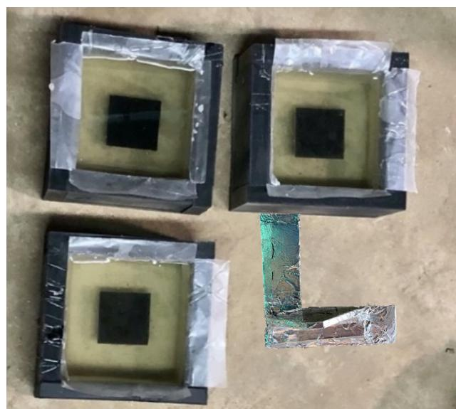
**Figure 2.** The liquid ballistic gel in the wooden frame showing the  $5 \times 5$  cm wood chamber piece and the parchment paper underneath the ballistic gel. The bottom right shows a picture of the L-shaped jig used to find the centre of each mould.
