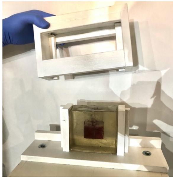
**Figure 4.** Ballistic gel mould with blood placed in its securing gel block.
