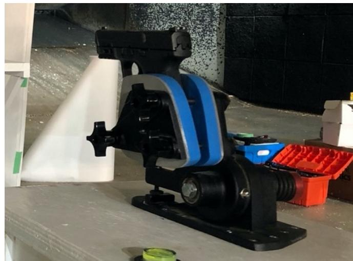
**Figure 6.** Ransom rest mechanism used to hold the gun at a controlled height and level.
