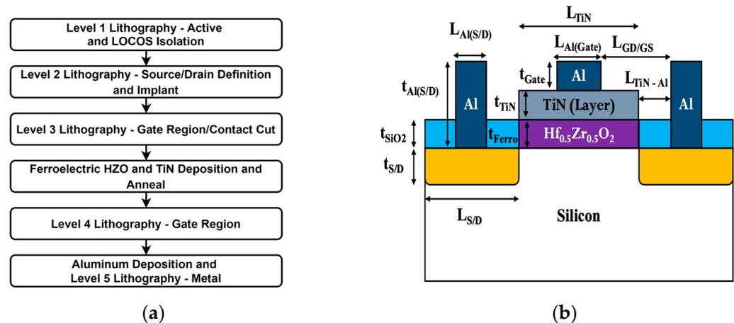
**Figure 2.** (a) Process flow for the fabrication of FeFETs, and (b) Schematic diagram of a fabricated FeFET.
