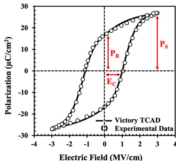
**Figure 4.** Measured and simulated polarization-electric field hysteresis loop of TiN/10 nm HZO/TiN capacitor.
