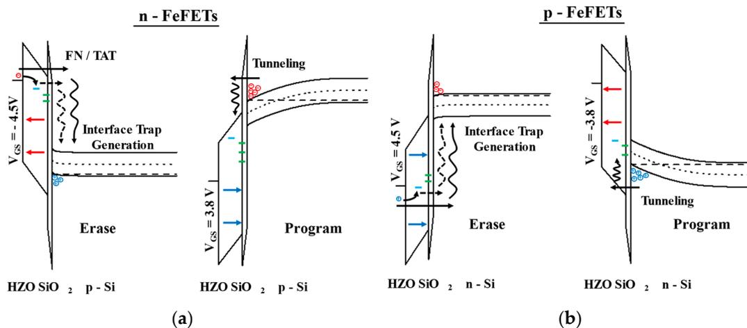
**Figure 10.** Band diagrams under erase and program conditions for (a) n-FeFETs, and (b) p-FeFETs. Red and Blue Arrows ( $\rightarrow$ / $\rightarrow$ ) in the SiO<sub>2</sub> dictate the orientation of the polarization field, the Black Arrow ( $\rightarrow$ ) dictates the tunneling direction, while the green and blue symbols ( $-/-$ ) represent the traps in bulk HZO and HZO/IL interface.
