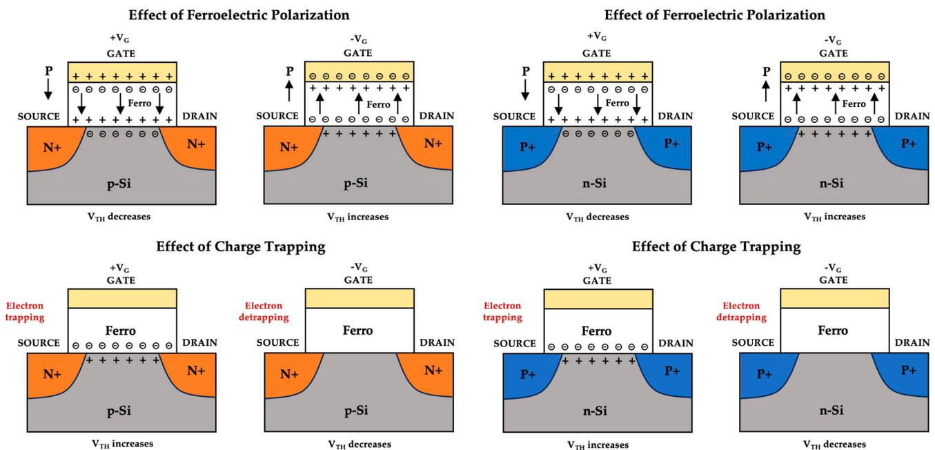
**Figure 1.** Effect of polarization switching and charge trapping on the threshold voltage shift in MOSFETs.
