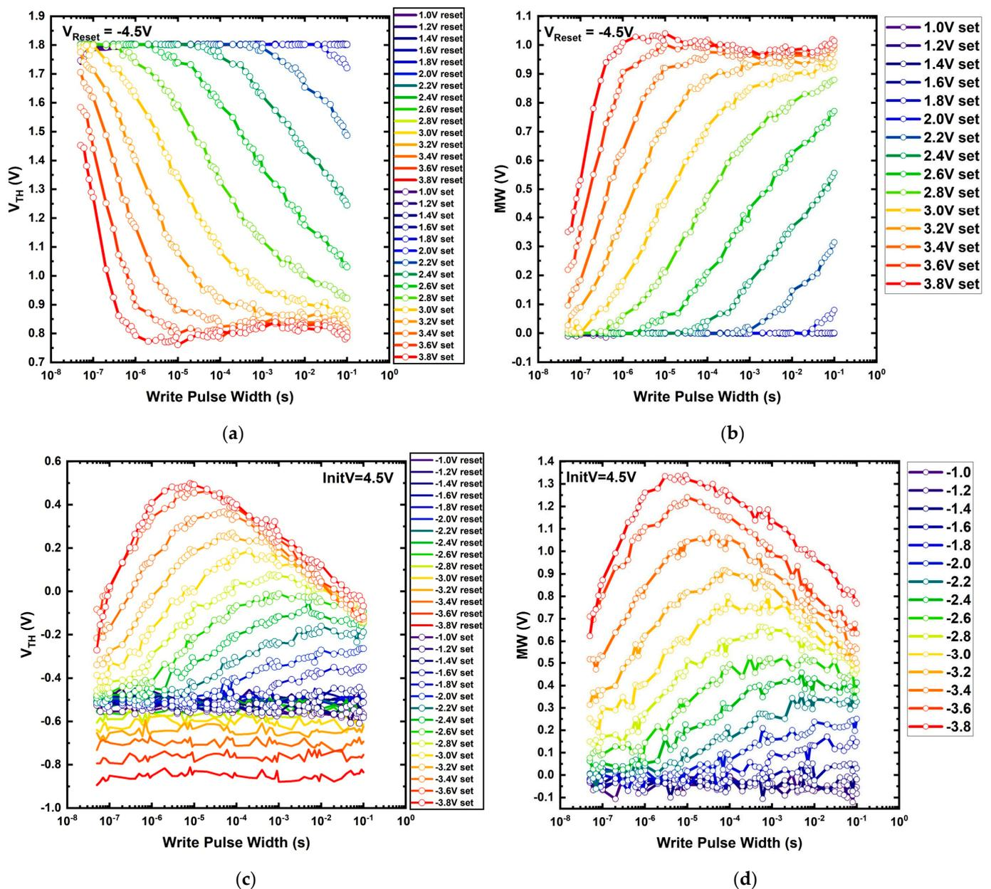
**Figure 7.** Partial polarization switching by varying the pulse width: (a) Gradual tuning of  $V_{TH}$ , and (b) MW for n-channel, (c) Gradual tuning of  $V_{TH}$ , and (d) MW for p-channel by increasing the width of the program pulse.
