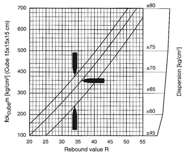
**Figure 4.** Characteristic curve for concrete and rebound hammer model: N/NR [11].
