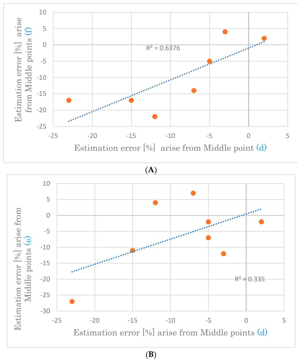
**Figure 12.** Error in compressive strength estimation. (A) Closeness of estimation error between middle points (d) and (f); (B) Closeness of estimation error between middle points (d) and (e).
