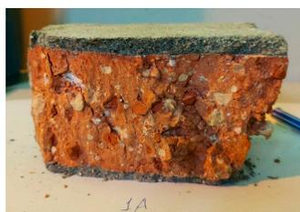
**Figure 1.** Internal microstructure of the *historical* brick.
