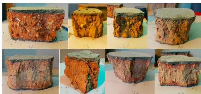
Figure 8. Satisfactory failures of specimen.
