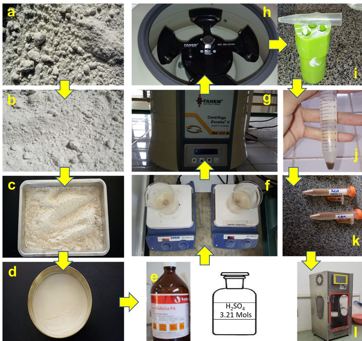
Figure 2. Steps for obtaining aqueous suspensions of PRSP nanostructures: (a) wet PRSP sample collected at the processing plant; (b) PRSP sample air-dried at room temperature; (c) oven-dried PRSP sample; (d) PRSP after drying, sieving, and particle size classification (bottom fraction of the sieve series); (e) sulfuric acid (analytical grade) diluted in distilled water to obtain the desired molar concentration; (f) acid hydrolysis of PRSP at the specified molar concentration for 5 days under constant stirring and temperatures; (g) centrifugation of the hydrolyzed suspension; (h) centrifuge rotor (tube holder); (i) centrifuge tube placed in the rotor during operation; (j) centrifuged sample showing phase separation according to density, with precipitate (brown phase) and supernatant (white phase); (k) colloidal suspensions (precipitate) containing starchy nanostructured after five washing cycles with (3.21 mols system), and (l) High-power sonicator used for nanostructure dispersion.
