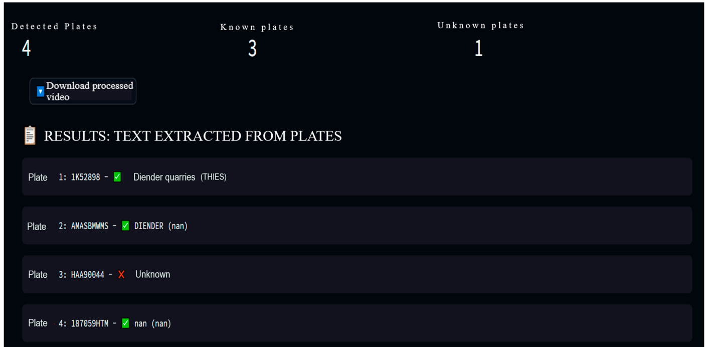
Figure 11. OCR extraction and registry verification. The side panel displays the canonical string and candidate scores, while the registry view confirms plate validity; together, they form the auditable evidence attached to each fused passage-plus-plate record.
