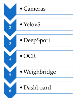
Figure 2. Reconciliation workflow linking detection and weighbridge data. Cameras: 1920 \times 1080 @ 25 fps, 8 mm focal length, 3.2 m above ground, lateral angle \approx 30^\circ .
