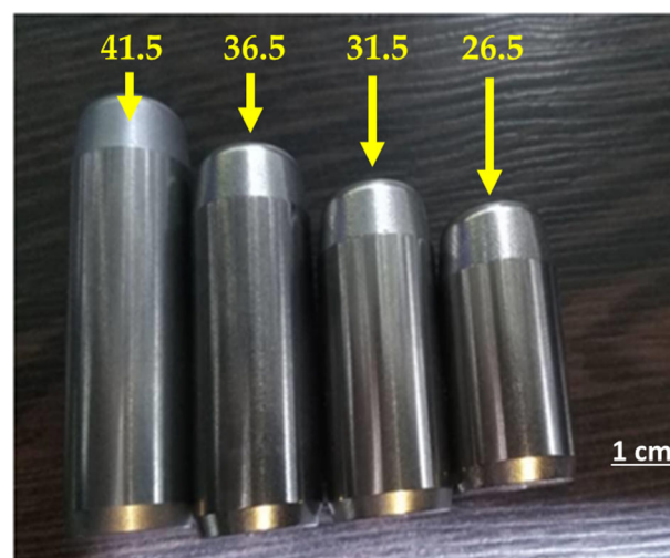
Figure 9. Sizes of replaceable studs: 26.5, 31.5, 36.5, 41.5.
