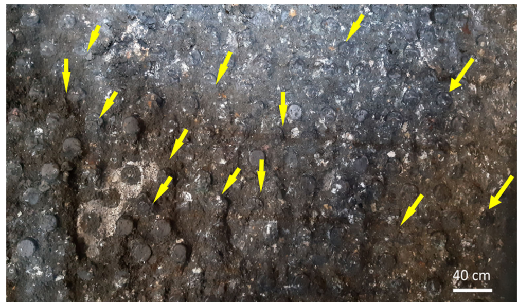
Figure 10. Failure to replace broken studs and continuation of the crushing operation. Arrows indicate regional failures.
