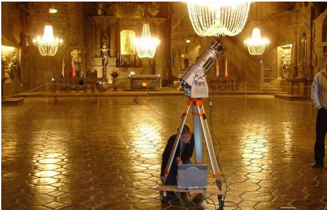
Figure 8. Measurement with a Riegl pulse scanner [17].
