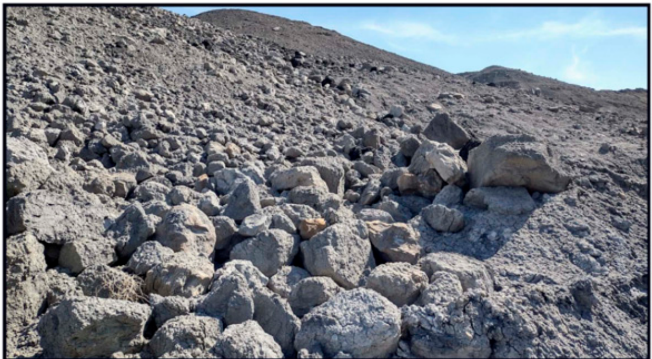
Figure 6. View of the particle size variability in waste rock generated at the Cordero Rojo Mine in the Powder River Basin, Wyoming, USA. Waste rock can range from clays to boulders.
