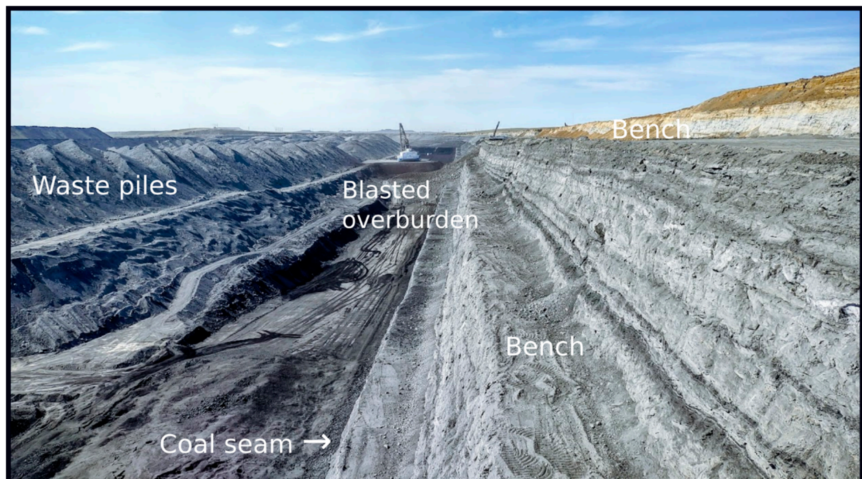
Figure 3. Removal of overburden and waste generation during open-pit coal mining at the Cordero Rojo Mine, Powder River Basin, Wyoming, USA (Martin and Langman [31]).
