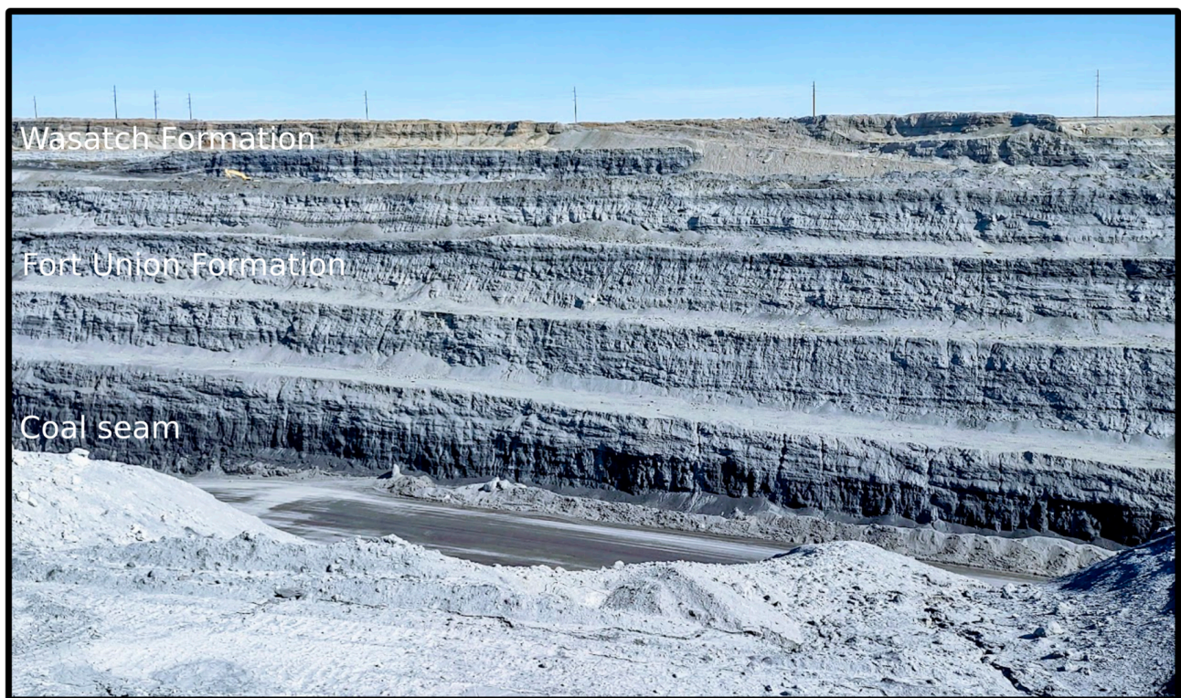
Figure 5. Overburden and coal seam at the Cordero Rojo Mine, Powder River Basin, Wyoming, USA (Martin and Langman [31]).
