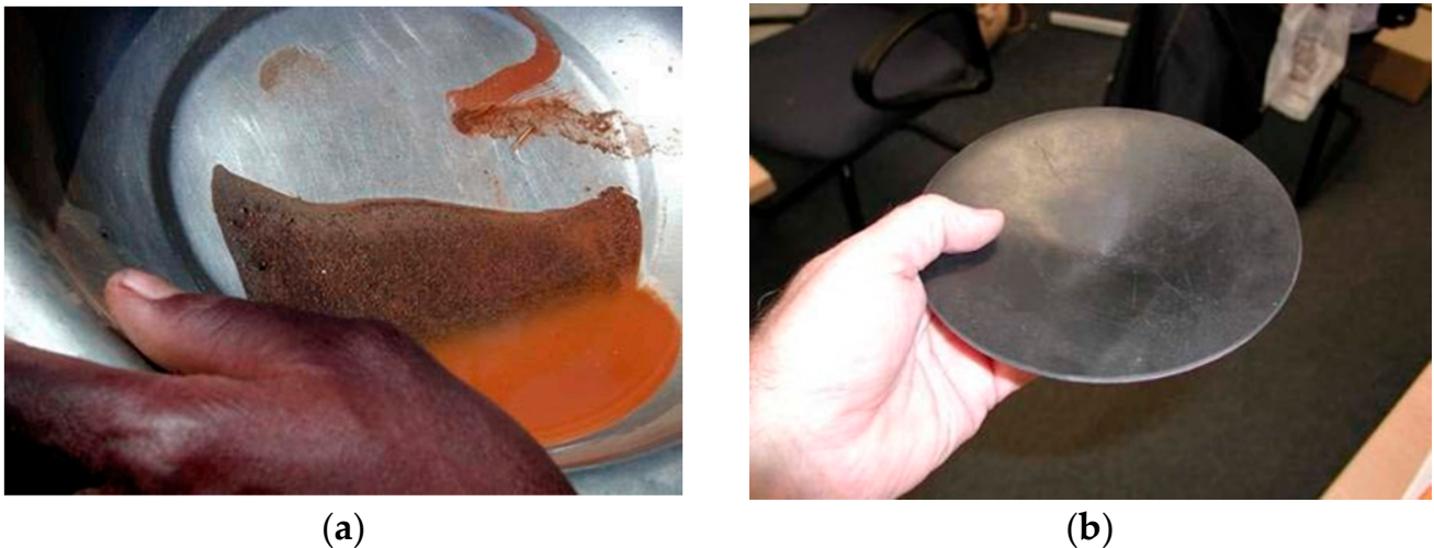
Figure 9. (a) Aluminum kitchen bowl used as a gold pan (Sudan); (b) small rubber-coated batea for testing the ore (Peru) [50].
