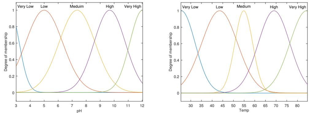
Figure 4. Memberships for pH and temperature.
