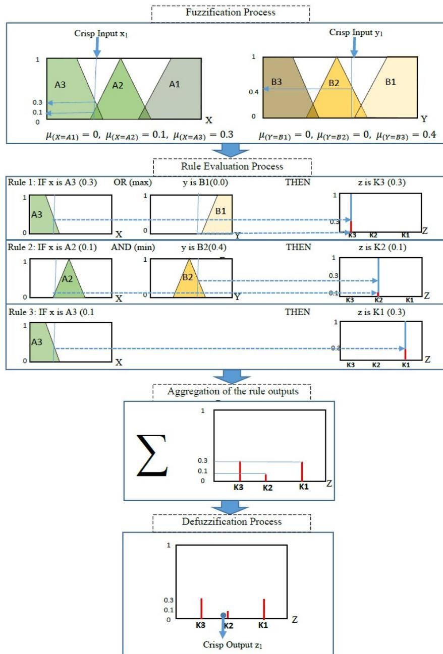
Figure 1. The structure of Sugeno fuzzy inference.
