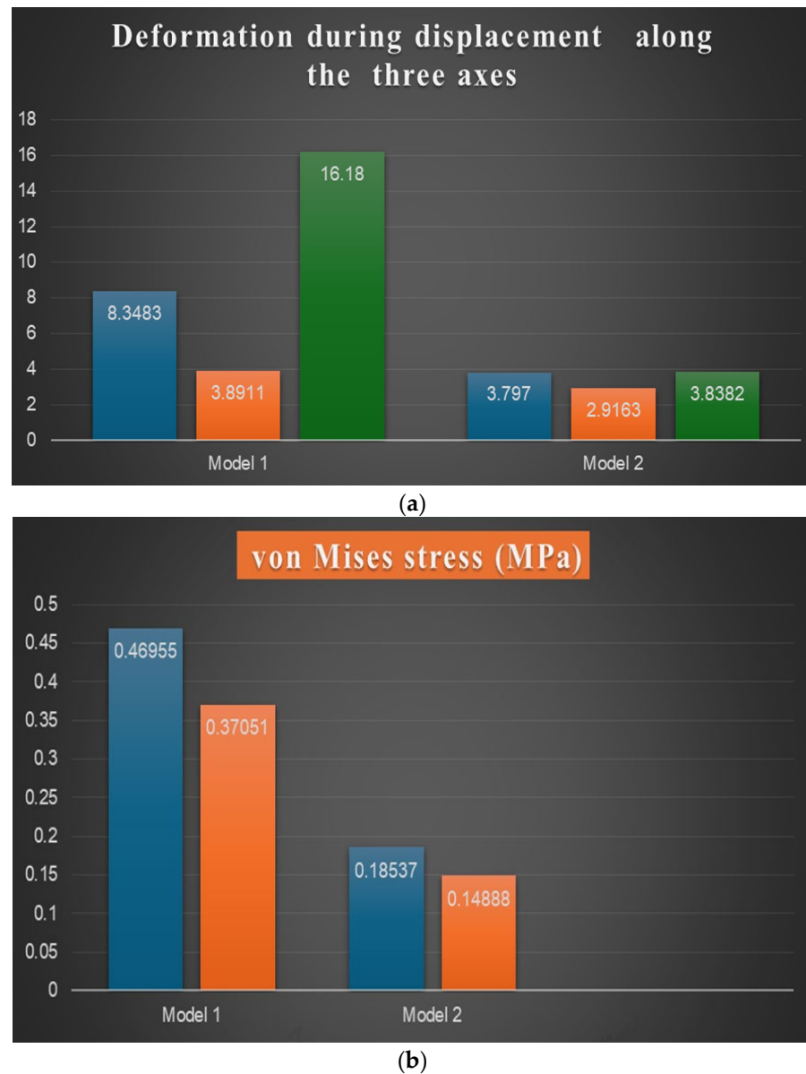
Figure 7. Graphical representations of (a) the displacement values (where blue represents the X-axis, orange the Y-axis, and green represents the Z-axis displacements) and (b) the von Mises stress for the mesial root (in blue) and for the distal root (in orange).
