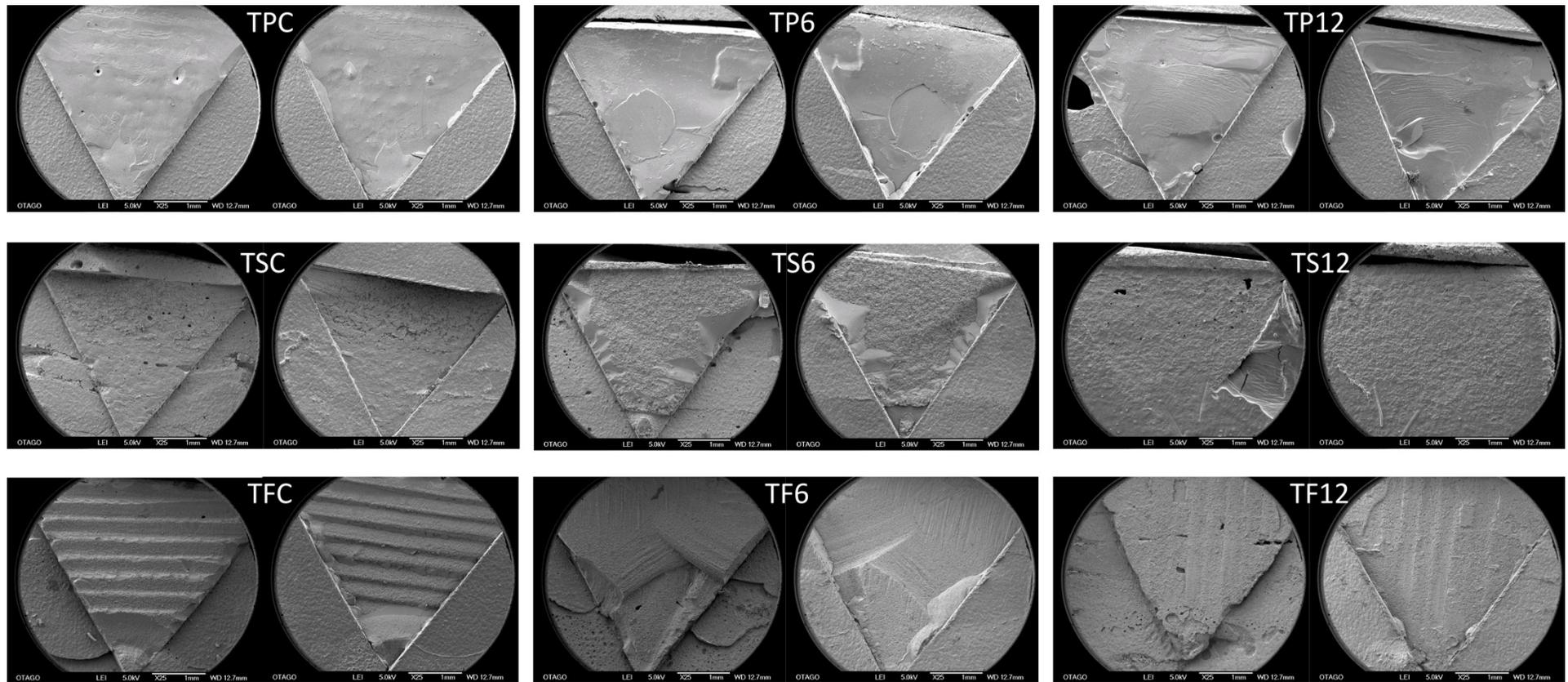
**Figure 6.** Representative SEM images ( $\times 25$  magnification) of one specimen per group (*T*: Telio CAD, *P*: Pala-Creative, *S*: SR Nexco, *F*: Ceramage, *C*: control, 6: 6 months, 12: 12 months). On the left-hand side of each slide, the composite is shown, on the right-hand side of each slide, CAD material is shown.
