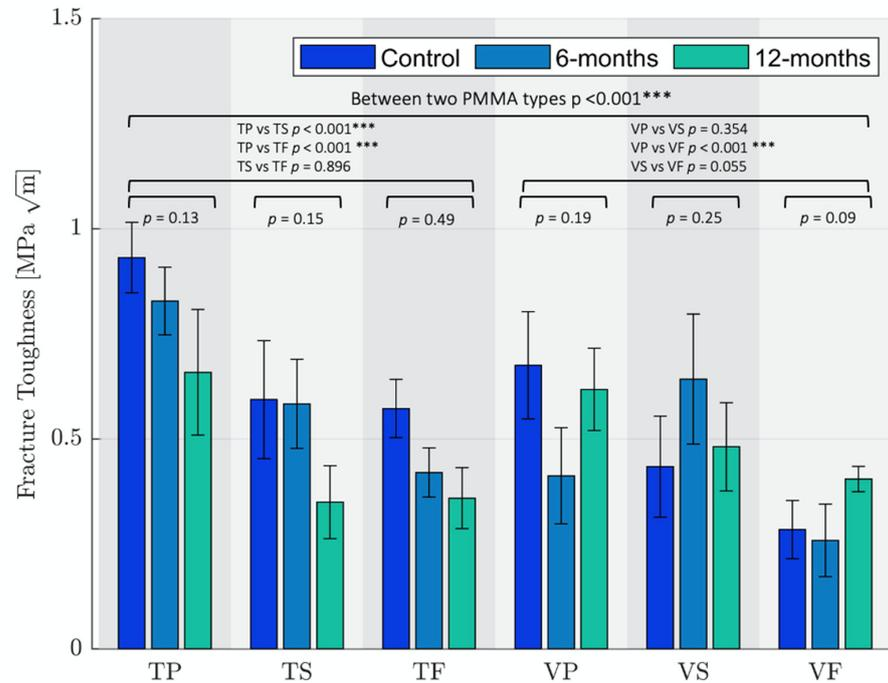
**Figure 3.** Fracture toughness of all sample groups representing control, 6 months and 12 months. The vertical lines represent 95% Confidence Interval ranges for Tukey’s pairwise comparisons. \*\*\* indicates a statistical significance level  $p < 0.001$ .
