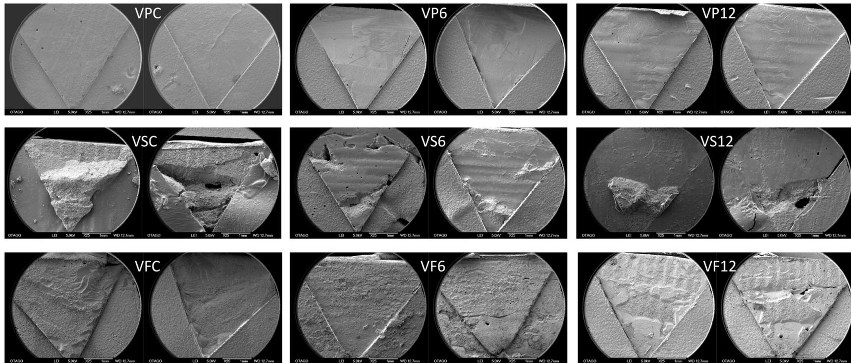
**Figure 5.** Representative SEM images ( $\times 25$  magnification) of one specimen per group (*T*: Telio CAD, *V*: Vivodent CAD, *S*: SR Nexo, *F*: Ceramage, *C*: control, 6: 6 months, 12: 12 months). on the left-hand side of each slide, the composite is shown, on the right-hand side of each slide, CAD material is shown.
