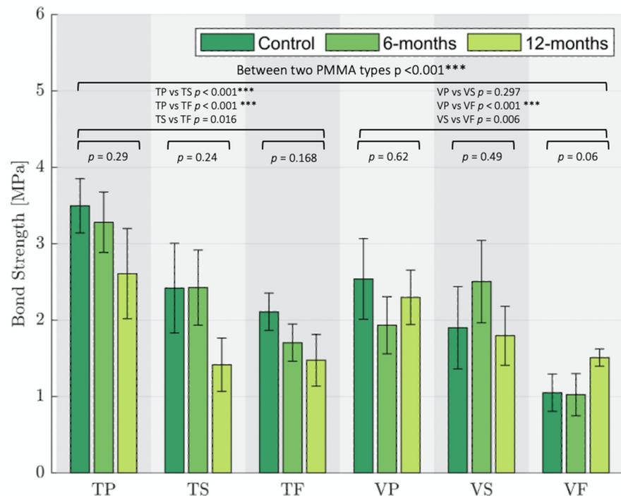
**Figure 4.** Flexural bond strength (MPa with mean bars) of all sample groups representing control, 6 months and 12 months. The vertical lines represent 95% Confidence Interval ranges for Tukey’s pairwise comparisons. \*\*\* indicates a statistical significance level  $p < 0.001$ .
