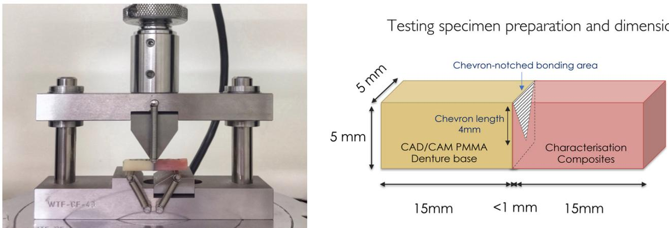
**Figure 2.** Images showing the chevron-notch three-point bend flexure bond test set up and specimen dimension (Chevron notch dimension is an equilateral triangle with a side of 5 mm).
