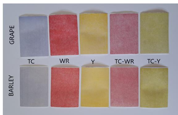
**Figure 1.** Two thermochromic mixtures prepared by adding conventional UV WR and Y offset-printing inks to the TC system in ratio 30:70, producing the effect of magenta (TC-WR) and green (TC-Y).
