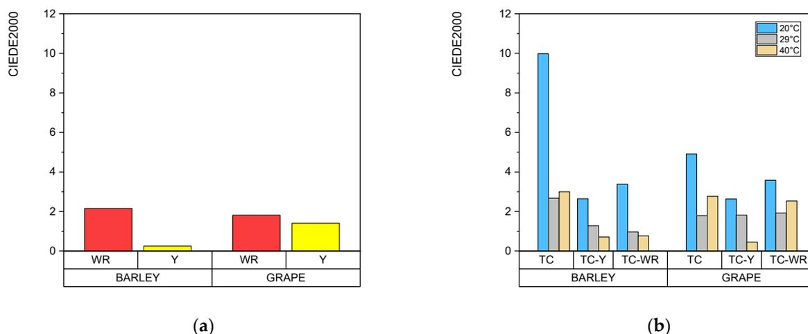
**Figure 6.** CIEDE2000 of the print after UV aging test of prints made from (a) conventional inks and prints made from (b) TC ink and mixture of TC and conventional inks.
