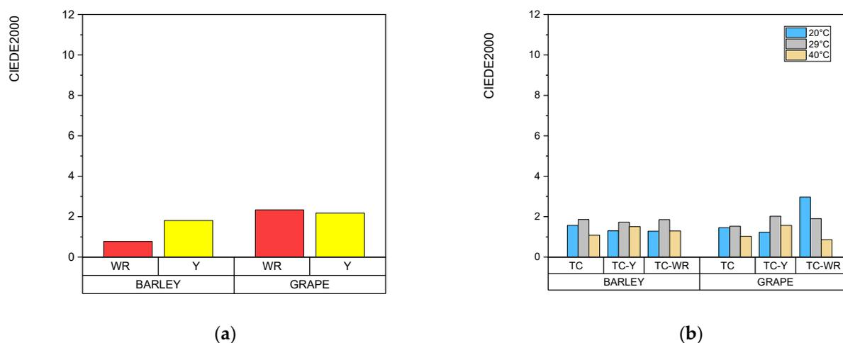
**Figure 2.** CIEDE2000 of the prints after rub resistance test of (a) prints made from conventional inks and (b) prints made from TC ink and mixture of TC and conventional inks.
