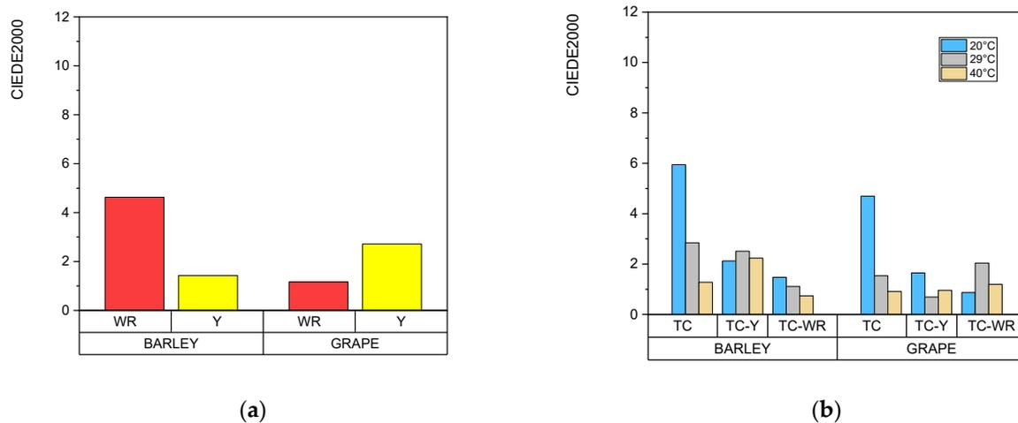
**Figure 3.** CIEDE2000 of the print after water resistance test of (a) prints made from conventional inks and (b) prints made from TC ink and mixture of TC and conventional inks.
