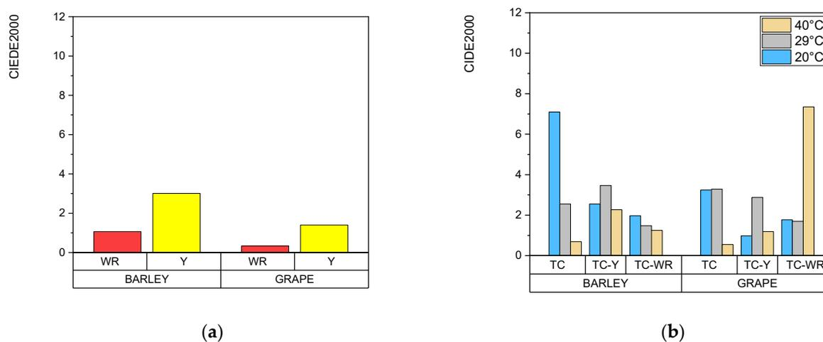
**Figure 4.** CIEDE2000 of the prints after ethanol resistance test of (a) prints made from conventional inks and (b) prints made from TC ink and mixture of TC and conventional inks.
