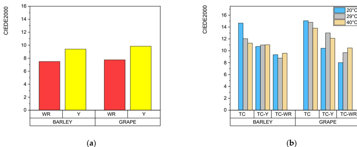
**Figure 5.** CIEDE2000 of the print after oil resistance test of (a) prints made from conventional inks and (b) prints made from TC ink and a mixture of TC and conventional inks.
