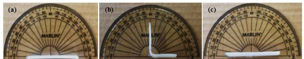
**Figure 5.** Shape memory behavior of the 3D-printed PLA specimens: (a) initial PLA specimen at 180°; (b) programmed specimen (the specimen was heated in a conventional oven at 80 °C for 1 min, then programmed at 90°, and finally cooled to room temperature); (c) specimen is reverted to the oven at 80 °C for shape recovery.
