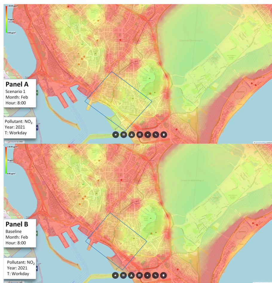
Figure 7. NO 2 heatmap for February 2021: Panel (A) shows the proposed Scenario 1—Viale Colombo deactivation—with traffic rerouted, while Panel (B) depicts the situation under current traffic conditions (Baseline Scenario). The highlighted area (blue boxes) indicate the waterfront section most affected by the changes.
