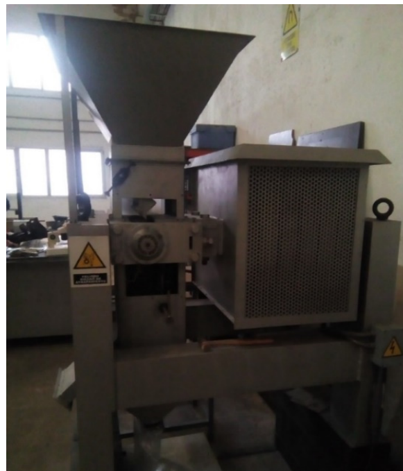
Figure 1. Induced rotor high intensity magnetic separator. Felemamg facilities in Gijón, Asturias, Spain.
