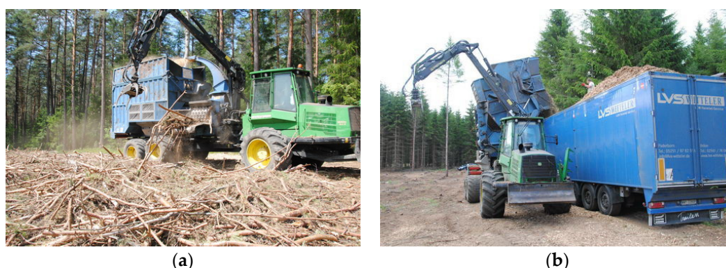
Figure 1. The BRUKS 805 CT chipper: (a) chipping of logging residues; (b) unloading.
