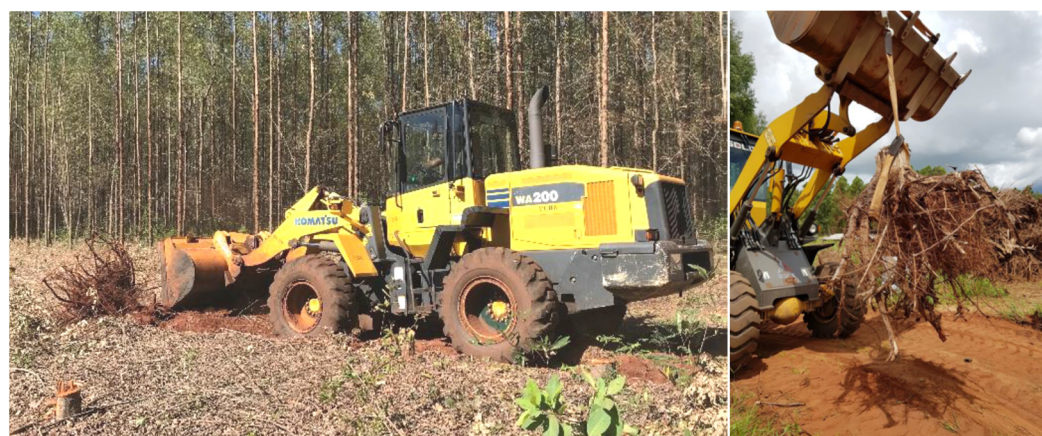
Figure 1. Stumps pulled out of the ground and weighted with a portable dynamometer.
