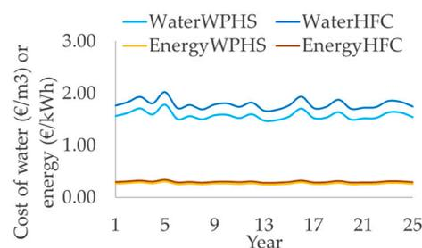
**Figure 3.** Cost of water and cost of energy for WPHS and HFC for 25 years.
