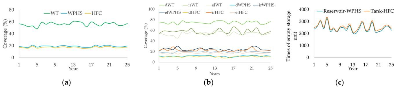
**Figure 2.** Coverage percentage per energy source for 25 years: (a) total coverage of demand per energy source; (b) coverage per demand per energy source; and (c) times of empty storage unit (upper reservoir or hydrogen tank).
