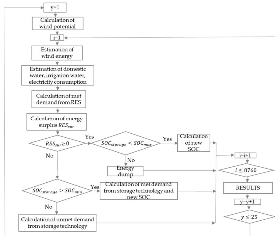
Figure 1. Flow chart of the operation of the HRES.
