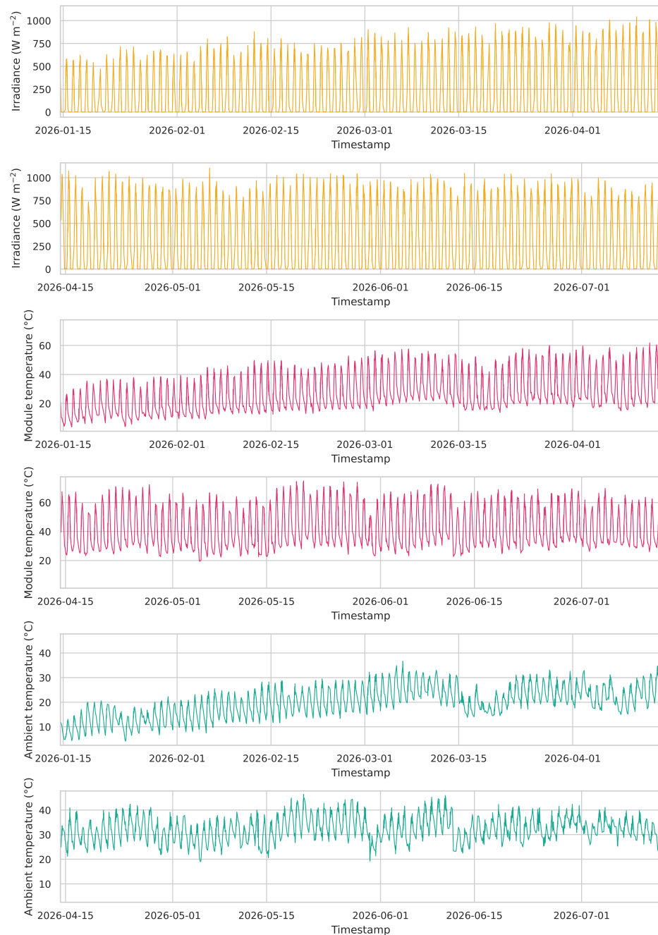
Figure 5. Measured irradiance, module temperature and ambient temperature over the complete Lahore plant dataset time axis.
