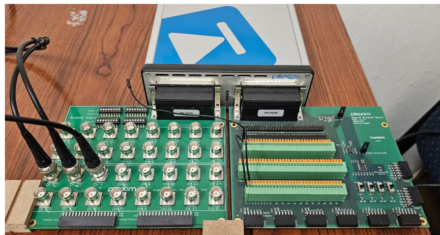
Figure 9. RTBox platform used for real-time hardware implementation.
