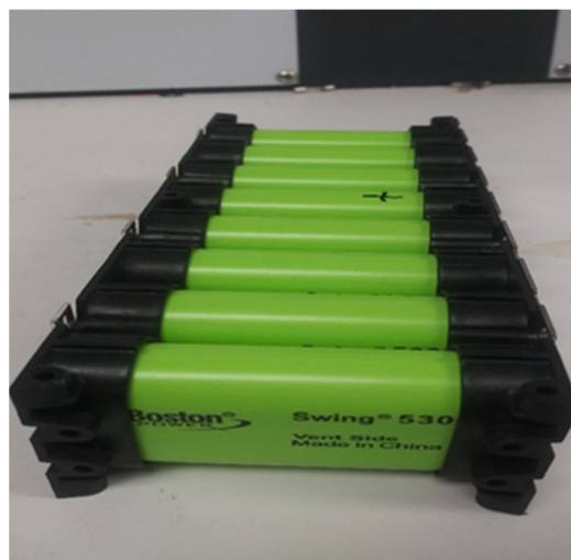
Figure 10. 24S battery using cells as shown in Figure 9.
