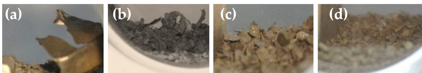
Figure 1. Specification of the hydrogenated magnetic material. (a) Non-decomposed coating: large coating areas remain unbroken, but are deformed by the volume expansion of the hydrogenated magnetic material, resulting in coating carcasses. (b) Single flakes: formed when the coating is not disintegrated by H_2 but is peeled off in flakes. (c) Mixed flakes: caused by better adhesion of the coating to the magnetic material and not by cohesion of the coating itself. (d) Disintegrated coating: small flakes caused by low cohesion or by reaction with H_2 .
