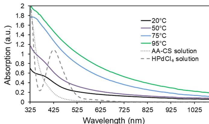
**Figure 1.** The UV-Vis absorption spectra of AA-CS solution,  $\text{HPdCl}_4$  solution, and PdNPs solutions.
