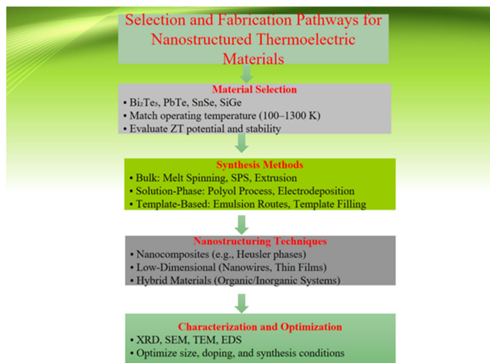
Figure 4. Selection and fabrication pathways for nanostructured thermoelectric materials.
