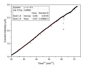
**Figure 2.** Behavior of the current intensity vs.  $t^{\frac{1}{2}}$  during water adsorption by a fully dehydrated clinoptilolite sample.
