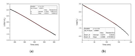
**Figure 3.** Fitting of the current intensity data by the pseudo-first-order irreversible model of Lagergren (**a**); and behavior of the relative current intensity logarithm during water desorption from a natural clinoptilolite sample (**b**).
