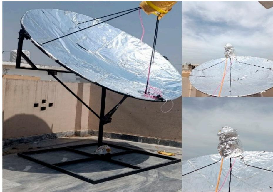
Figure 2. Experimental setup for solar parabolic dish.
