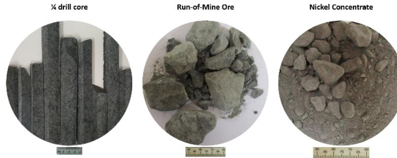
**Figure 1.** Samples of drill core, run-of-mine ore (ROM), and nickel concentrate.
