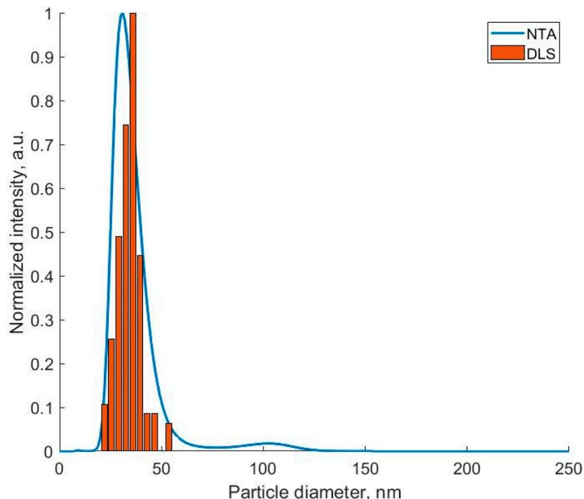
**Figure 2.** Particle size distributions for sample 1 of gold nanoparticles measured using NTA (blue) and DLS (orange) techniques.
