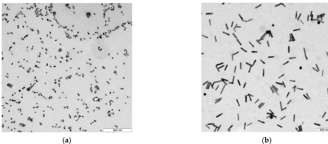
**Figure 1.** TEM images of gold nanorods' diluted samples: (a) aspect ratio of 2; (b) aspect ratio of 6. It should be mentioned that there were also detected quasi-spherical particle impurities, especially in samples with aspect ratio more than 3.
