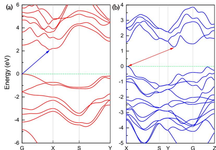
**Figure 2.** The band structure of (a) the monolayer and (b) the bulk of GeSnS2.
