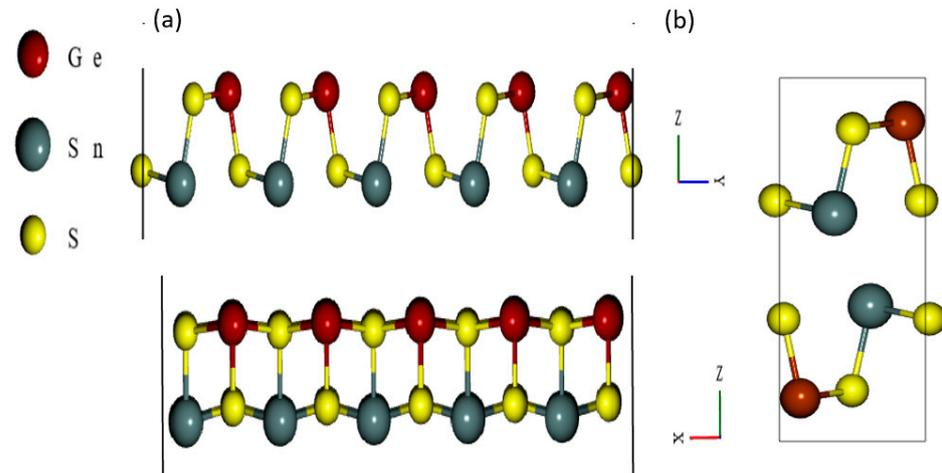
**Figure 1.** (a) Top and side monolayer views; (b) the bulk structure of GeSnS2.
