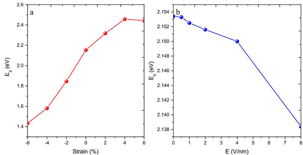
**Figure 3.** The variation of band gap energy with (a) strain (red curve) and (b) an electric field (blue curve).
