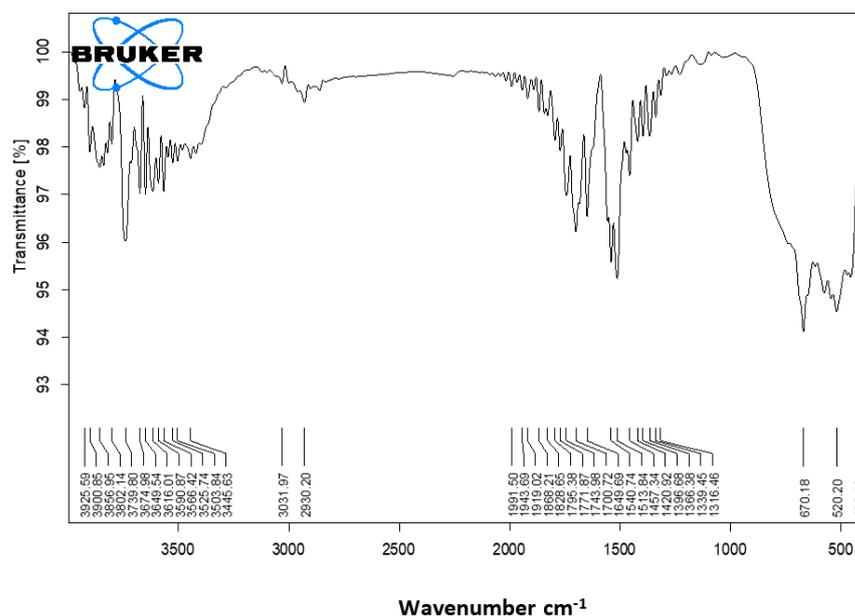
**Figure 3.** FT-IR spectrum of TiO<sub>2</sub> NPs.
