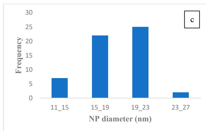
**Figure 5.** (a) FE-SEM images and (b) EDX image of synthesized TiO<sub>2</sub> NPs, and (c) Histogram of TiO<sub>2</sub> NP size distribution.
