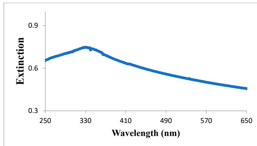
Figure 1. UV-Vis spectrum of the synthesized TiO<sub>2</sub> NPs.
