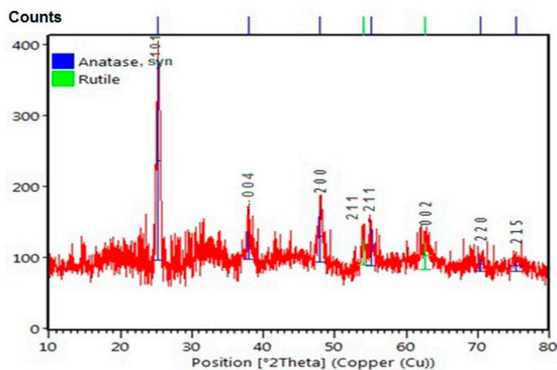
Figure 2. XRD pattern of TiO<sub>2</sub> NPs.
