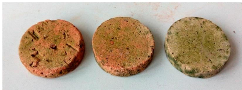
**Figure 7.** Samples of the Holešov-Žopy bricks covered by a biofilm layer of 0–1 cm, 1–2 cm and 2–3 cm (from left to right).
