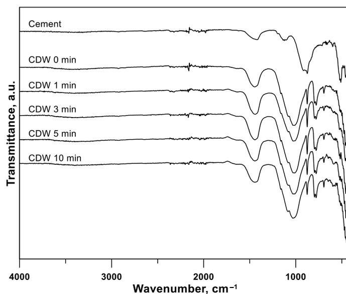
**Figure 1.** The FTIR spectra of the cement and ground CDW samples.
