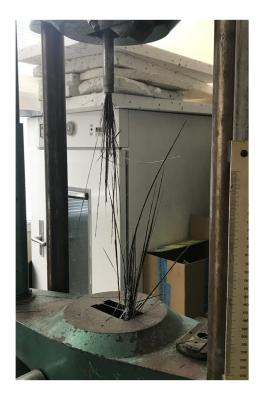
from the analysis. Nevertheless, elasticity moduli were calculated for these specimens. Figure 4 shows the typical mode of failure for the analysed specimens.
