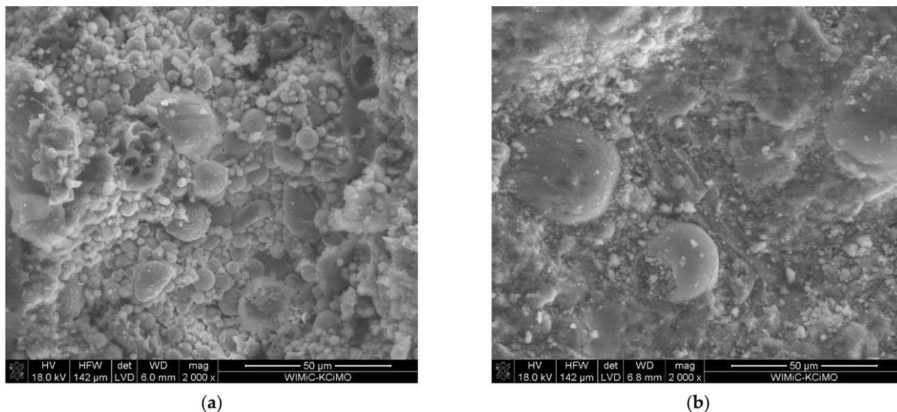
**Figure 3.** SEM micrographs of the 60PC-20GBFS-15SFA cement paste after (a) 2 days and (b) 28 days.
