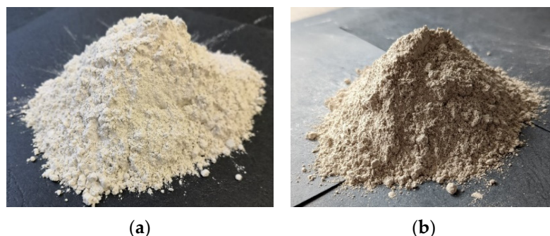
Figure 1. (a) Finely ground granulated blast furnace slag (GGBFS); (b) metashale (RON D460 HR).
