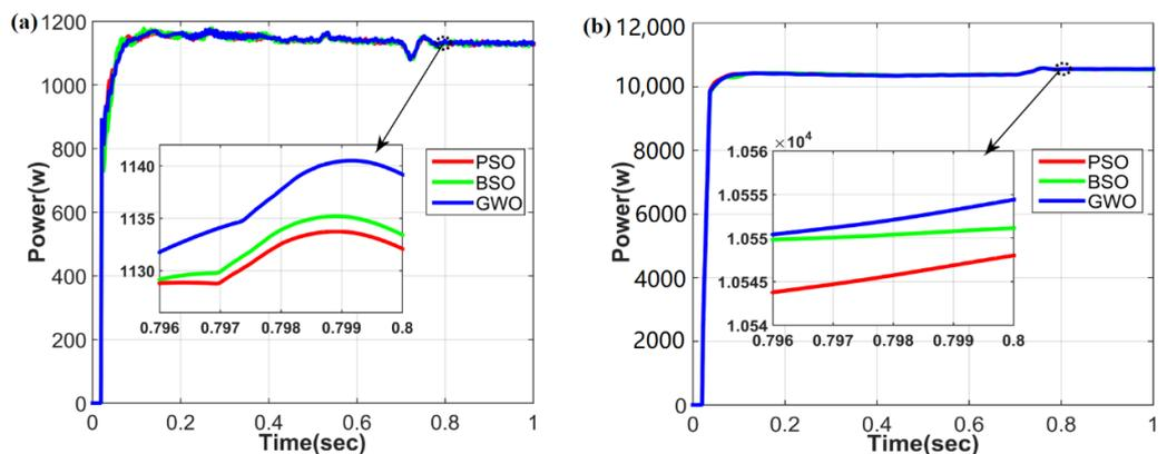
Figure 7. Comparison of powers under case-2 (a) PV Converter power (b) load power.
