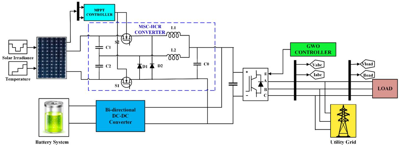
Figure 4. MATLAB Simulation Diagram of a grid-interfaced PV system.
