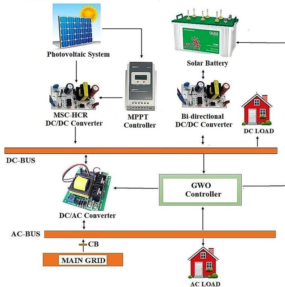
**Figure 1.** The architecture grid-interfaced PV system with GWO controller.
