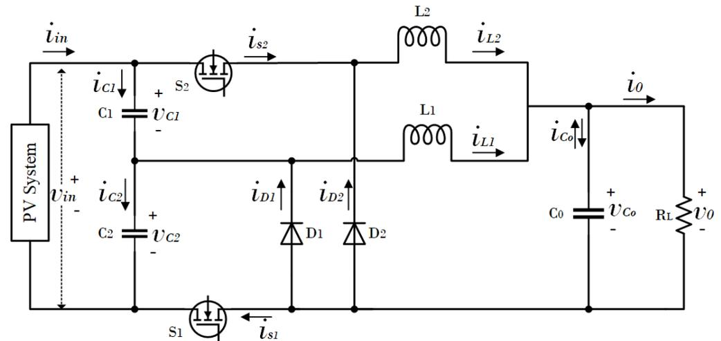
Figure 2. A circuit diagram of an MSC-HCR converter.
