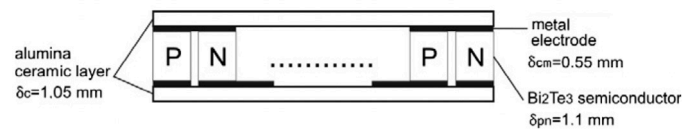
Figure 3. Schematic cross-sectional view of TEG module (Karabetoğlu et al. [12]).
