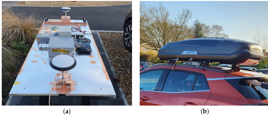
Figure 3. The physical hardware demonstrator. (a) Open demonstrator showing components and antennas. (b) Closed demonstrator in the car roof box.
