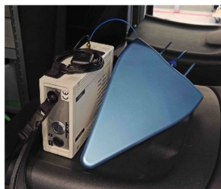
Figure 2. The battery-powered hand-held sensor (left) connected to a directional antenna (right). The user carries the sensor with a carrying strap and can access the user interface via a smartphone or tablet which connects to the sensor's WiFi access point.
