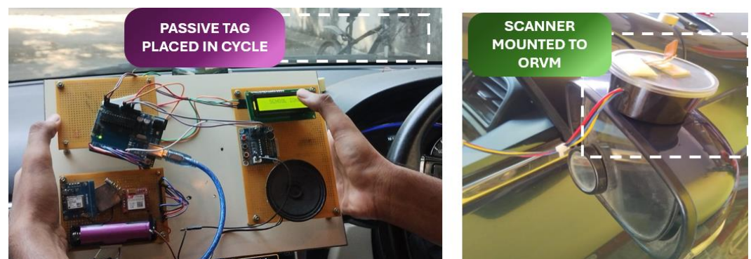
Figure 9. Real-time testing of the proposed system with the M7E-TERA-CB sensor.
