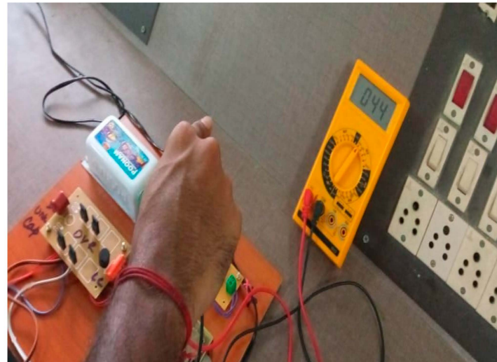
Figure 10. Voltage at output before using DVR.
