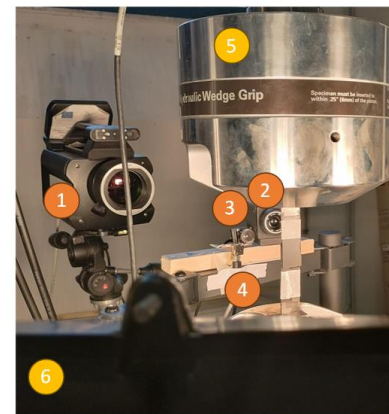
Figure 9. Experimental setup for thermographic and fatigue tests with technical and cost specifications.
