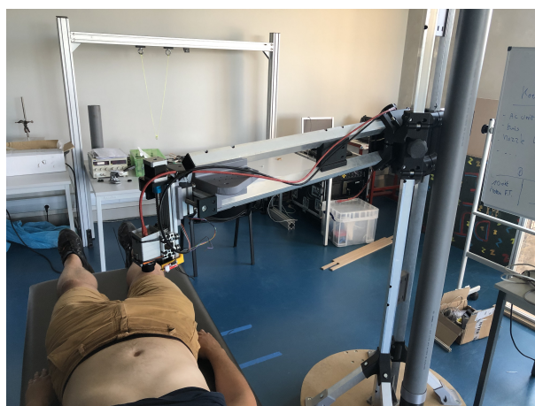
Figure 3. Image taken during skin tissue identification measurements. The thermal camera is mounted on the linear guide rails at the end of the mount arm. The mount enables the camera to be moved to any wanted location above the patients body, and the linear guide rails provide the possibility of keeping a fixed distance between the camera lens and the skin.
