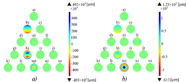
**Figure 4.** Aberration diagrams for (a) circular and (b) square apertures, with the piston and defocus aberrations eliminated. The values shown in the legend are the wavefront error in  $\mu\text{m}$ . The wavefront errors for study two are 400 times lower for the maximum error (in dark blue) and 804 times smaller for the minimum error (in dark red) than for the study one.
