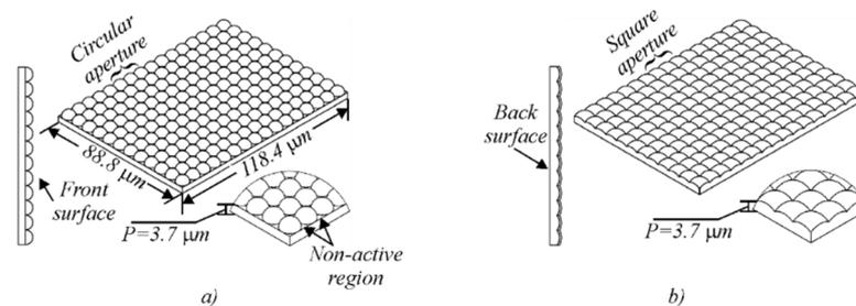
**Figure 2.** (a) Matrix of  $12 \times 16$  elements with the radius of curvature  $R_{a1} = 3.7 \mu\text{m}$  and circular aperture of  $D = 2R_{a1}$ . (b) Matrix of  $12 \times 16$  elements with the radius of curvature  $R_{a2} = 7.4 \mu\text{m}$  and square aperture with a side size of  $D = R_{a2}$ .
