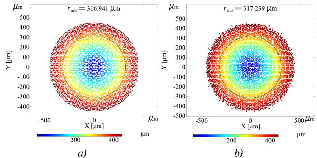
**Figure 3.** Spot images at the focal plane: (a) circular and (b) square aperture. The black circle indicates the RMS spot radius. The colors represent the lateral ray displacement from the point on the aperture to the position on the focal plane, and its contribution to wavefront and crosstalk error.
