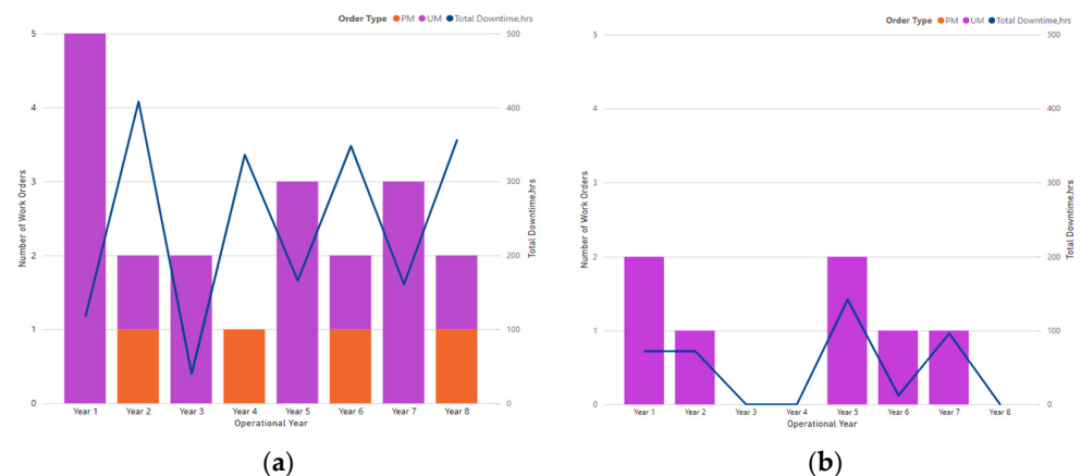
Figure 2. Annual maintenance distribution and downtimes before (a) and after data analysis (b).
