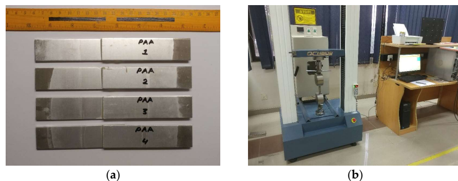
Figure 6. A visual representation of (a) manufactured SLJs, (b) testing of SLJs on UTM.
