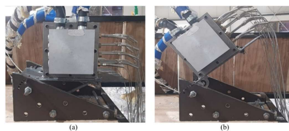
Figure 3. Illustrates (a) PCM enclosure at 0^{\circ} (b) PCM enclosure at 45^{\circ} .
